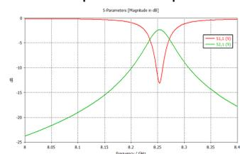
Figure 11: S-parameters of suspended stripline 1D line resonator filter
