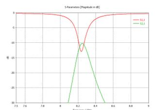
Figure 9: S-parameters of microstrip 1D line resonator filter
