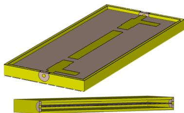
Figure 10: A perspective view and cross section of a suspended stripline filter
