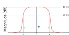
Figure 3: Bandpass filter frequency response
