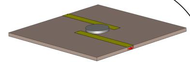
Figure 12: Dielectric Resonator Microstrip Filter
