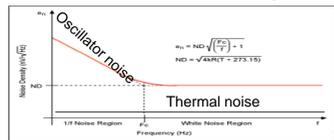
Figure 2: Oscillator noise
