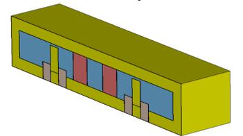
Figure 15: Dielectric Resonator Loaded Cavity Filter Cross Section
