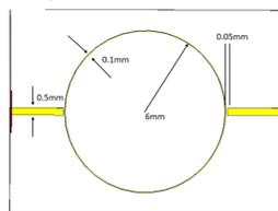
Figure 6: Microstrip filter. The ring resonator placed between two microstrip lines
