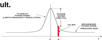
Figure 1: Signal oscillator spectrum
