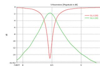
Figure 7: S-parameters of the filter above.
