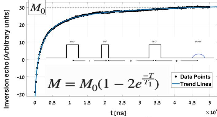
Fig 1: Inversion recovery (500gy Cs<sup>137</sup> exposure) by a Pulsed ESR fitted to the T<sub>1</sub> equation. T<sub>1</sub> = 43 ± 32 μs
