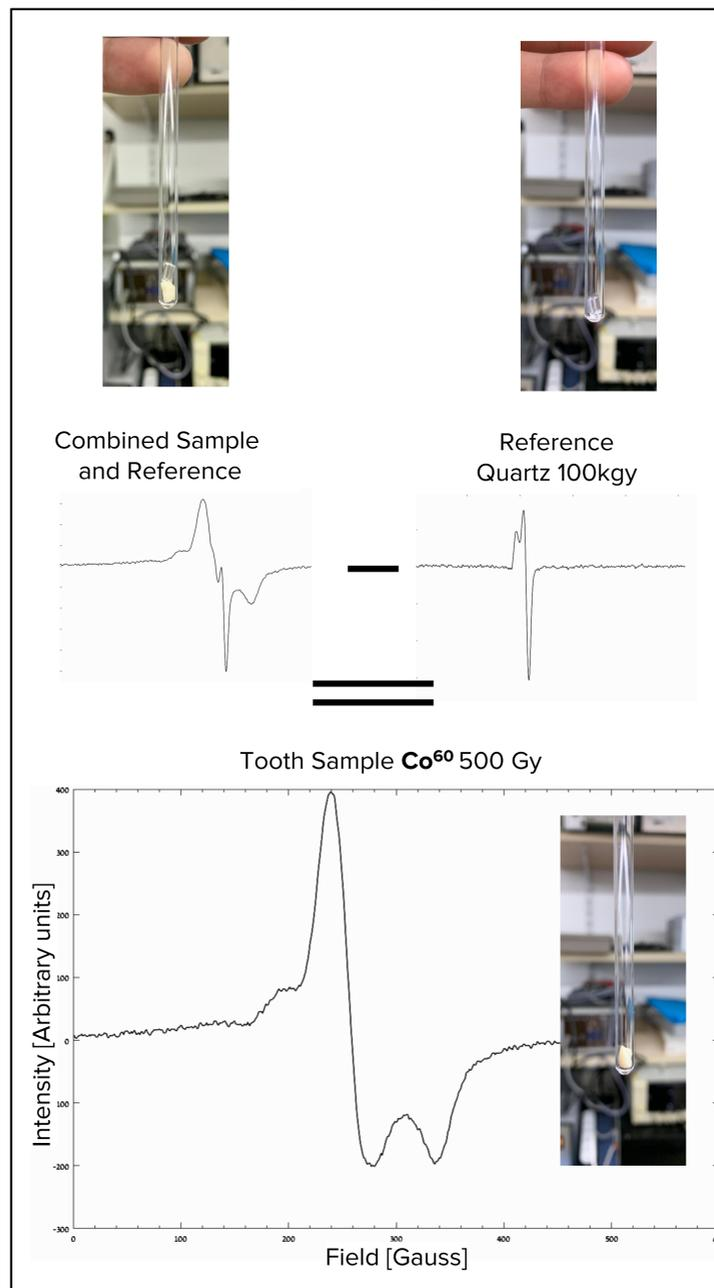
Fig 3. Upper - Pictures of the samples above their respective spectra. Lower - Continuous wave spectra along with pictures of the samples inside a tube. Double integral of the combined sample and reference on the top left minus the reference on the top right will give the double integral of the tooth sample. Comparing the tooth to a reference quartz with a known number of spins gives the tooth's number of spins.
