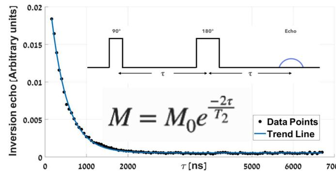
Fig 2: Echo decay (500gy Cs<sup>137</sup> exposure) by a Pulsed ESR fitted to the T<sub>2</sub> equation. T<sub>2</sub> = 788.7667 ns.
