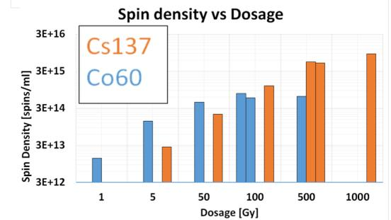
Fig 4. T<sub>2</sub> and Spin density vs radiation dosage results. Each bar represents a different tooth with the colors representing different radiation sources.
