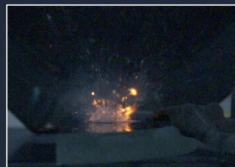
Fig. 10 - 79% T = 28 ms First flame that becomes a fire
