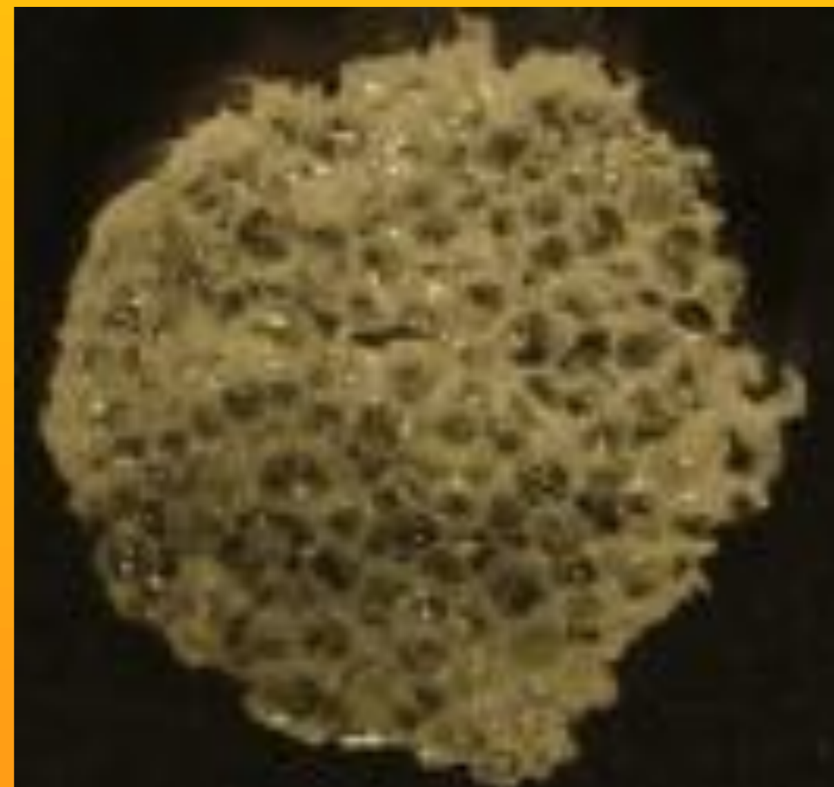
Fig 1. Synthetic PLLA/PLGA scaffold.
