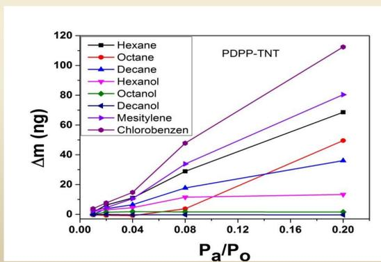
Figure 7. Mass shift for a QCM coated with PDPP-TNT
