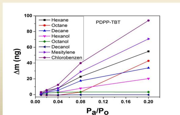
Figure 8. Mass shift for a QCM coated with PDPP-TBT
