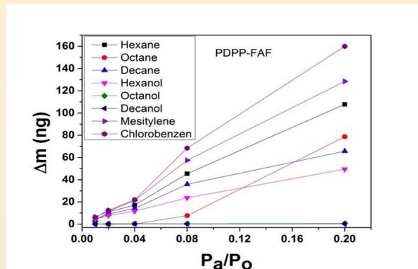
Figure 6. Mass shift for QCM coated with PDPP-FAF
