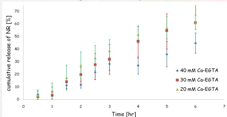
Figure 3: Cumulative release of NR from with alginate gels with different concentrations of calcium 20-40 mM and alginate concentration of 20 mg/ml.
