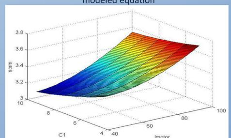
Figure 8: Norm vs. friction ( $c_1$ ) and inertia ( $I_{motor}$ )
