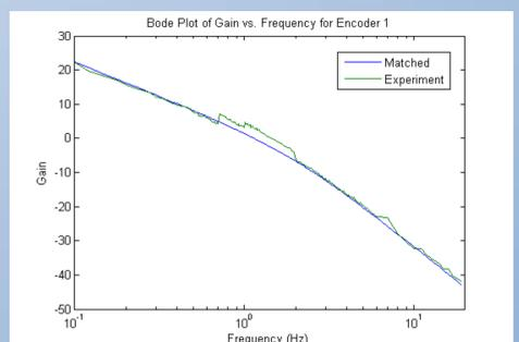
Figure 7: Bode plot for the motor with no load and the modeled equation
