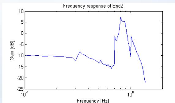
Figure 3: Bode plot for the robotic leg
