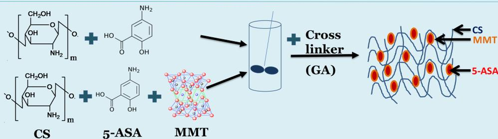
Figure 2. Schematic hydrogels preparation process
