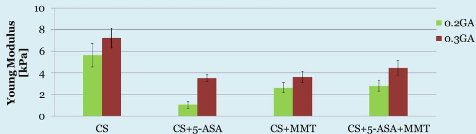
Figure 4. The mechanical strength of the hydrogels in different concentration of GA
