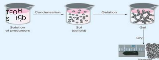
Figure 1. Sol-gel technique for biofilm matrix preparation.
